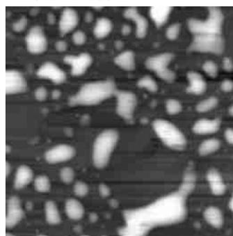
Fig. 4 An AFM image of autophobic dewetted molten MHPEO ( $M_n = 4700$  g/mol) droplets at 65
